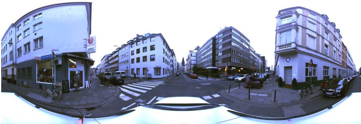
*A street view in Cologne taken with an omni-directional camera system. These photos, in combination with the products of remote sensing and engineering expert knowledge, provide a rapid assessment of the vulnerability of a building stock (photo by Marc Wieland, GFZ).*
